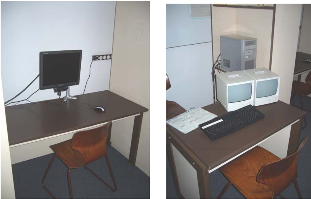
Figure 3: The Eyegaze Analysis System eye-tracker in the Lab. Left side: subject's desk with monitor and infra-red LEDs and cameras. Right side: the experimenter's desk with the control PC, eye control monitors and control keyboard.
